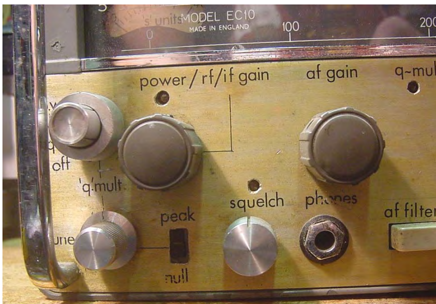
Left: close-up of the Q-Multiplier control section with the squelch control to the right next to the phones jack
